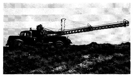
Spray Truck with Telescope Boom
